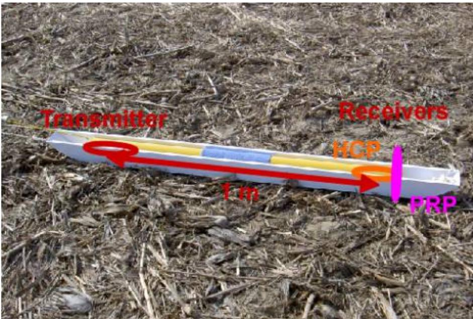
**Fig. 1. EM instrument with 1-m HCP and PRP arrays. (Photo: Dr. B. Allred)**
