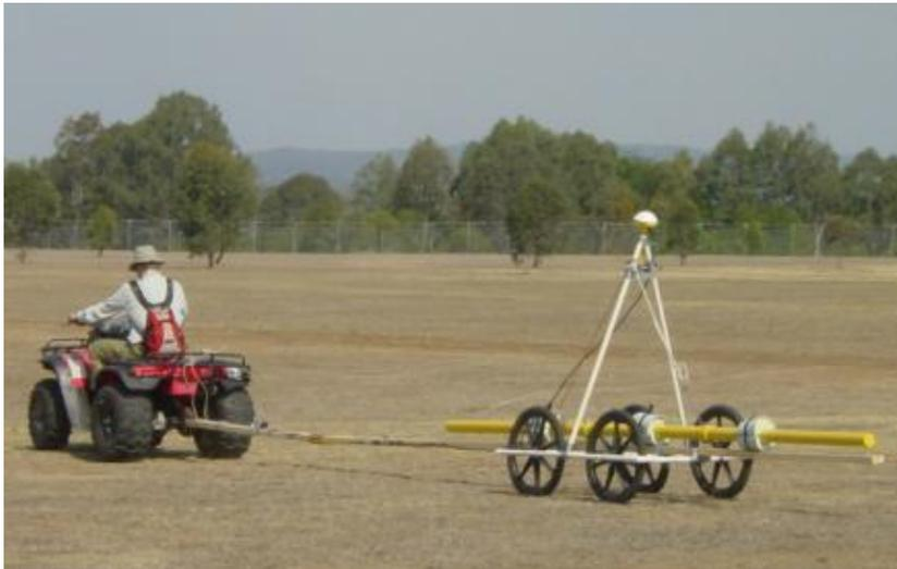
**Fig. 3. EM instrument on a cart with GPS.**
