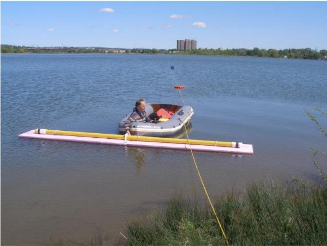
**Fig. 12. Survey line on lagoon, with EM instrument on raft.**
